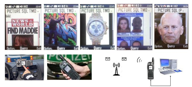
The Data Transmission works in Direct-Mode (DMO) or Infrastructure-Mode . In DMO and TMO the Data Transmission works via SDS4 – Textmessages. The JAVA Radio Terminal Application receives the Textmessages and converts the Text into a Picture. The Products are called **PICTURE SQL DMO** and **PICTURE SQL TMO**. The Control Room Dispatcher is able to send Pictures to single Users (ITSI's), too. For Offline-Reading Purpose the Pictures were saved permanently inside the EADS Radio Terminal.
